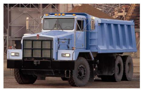
Kenworth C500, C508 & K108 Trucks can be fitted with 715-650 wheels on both Front Steer and Heavy Duty
