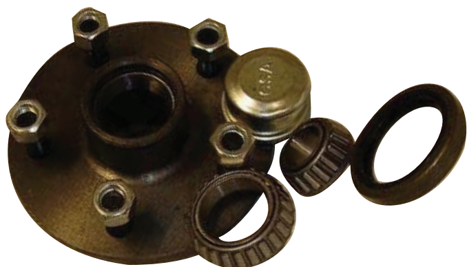
HUB COMPLETE HUB - PLAIN FINISH FORD - 5/4.5" - 5/114.3 PCD - 1/2" STUDS - 6" Dia FLANGE Part No. 860-B542i
