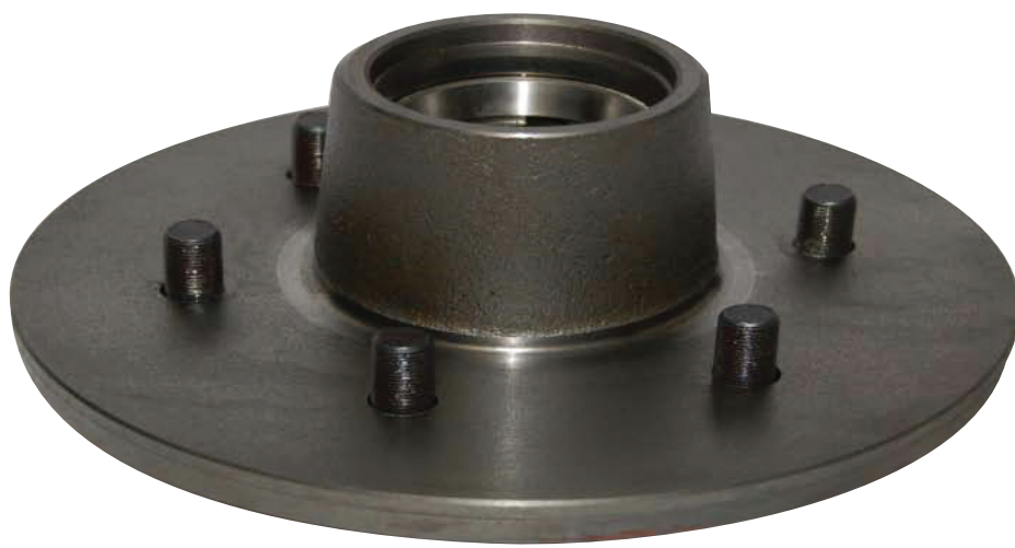
HUB - C TYPE - STUDDED & CUPPED ONLY LAND CRUISER 6 STUD - 6/5.5" - 6/139.7 PCD Part No. 860-ZC67
